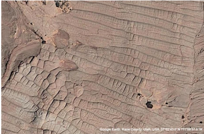
Figure 7. Satellite view of joint system in Aztec sandstone grading locally from hexagonal into orthogonal, pentagonal and linear patterns. Notice that finer scale systems exist within the main system suggesting that the energy potential that is minimized to form these patterns is non-convex.
